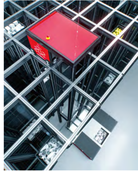
The new "auto store" will stock 52,000 boxes using a very space-saving system. The speciality about the system is the fact that the boxes aren't stored on shelves but in stacks of 16 boxes. The complex is managed by 15 computer-controlled robots that operate near the ceiling.
