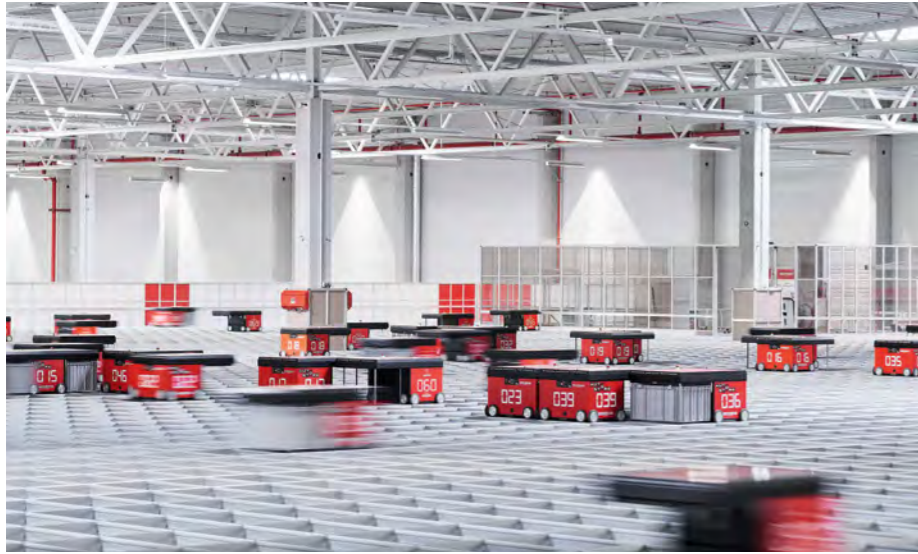
The new "auto store" will stock 52,000 boxes using a very space-saving system. The speciality about the system is the fact that the boxes aren't stored on shelves but in stacks of 16 boxes. The complex is managed by 15 computer-controlled robots that operate near the ceiling.
