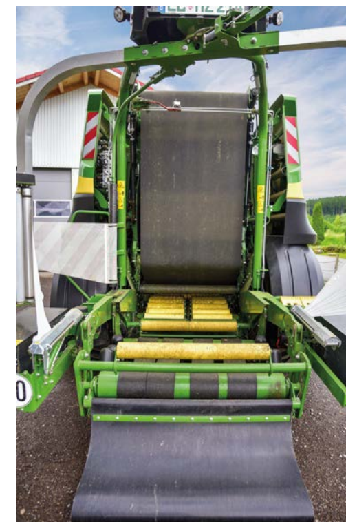
The mono belt design on the new KRONE CombiPack HDP means that rolling losses are almost completely prevented.
