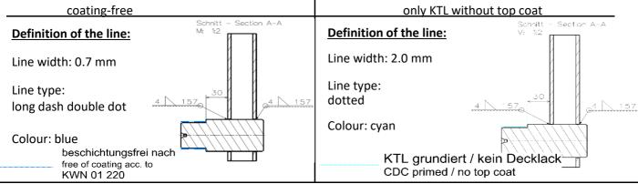
On parts with coating-free surfaces, the coating-free surfaces must be provided with corrosion protection agent. This also applies if the part has been delivered unpainted. Only means approved by KRONE may be used!
